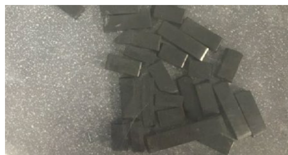
Figure 8: Broken piston rings on the NE (north east) cylinder.
