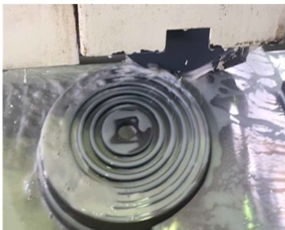
Figure 5: Using a surface grinding machine to get better flatness for sealing elements
