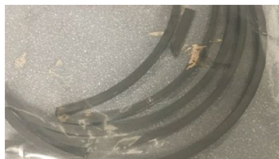
Figure 10: Piston rings on the SW (south west) cylinder came back heavily worn but mostly intact.
