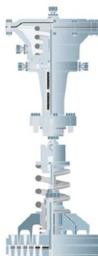
Figure 4: A pneumatic actuator of the type originally fitted to the operators compressor.
