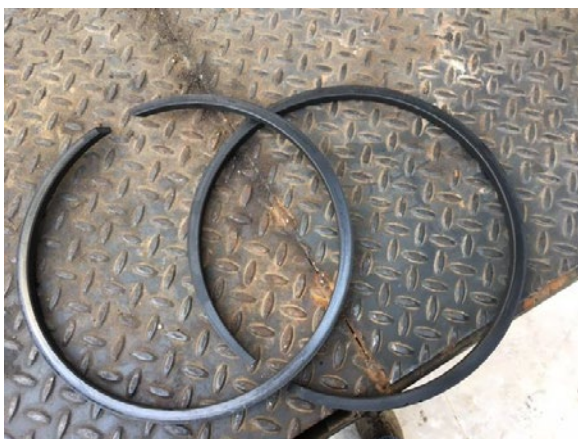
Figure 24: Piston rings with reduced radial thickness after the run indicating a heavy wear situation.
