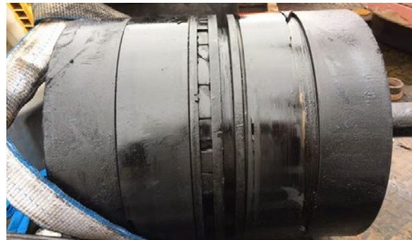
Figure 21: Piston after removal from cylinder in March 2018: Piston rings show signs of heavy wear and are broken into pieces. One rider band is broken as well. Particles trapped in viscous material on the piston of a recycle compressor can act similar to a lapping compound.
