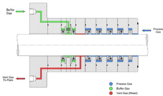
Figure 8: Low-friction buffer assembly positioned in a packing case
