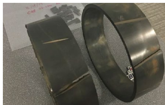
Figure 9: Both solid, shrunk-on rider bands on the NE cylinder were cracked.
