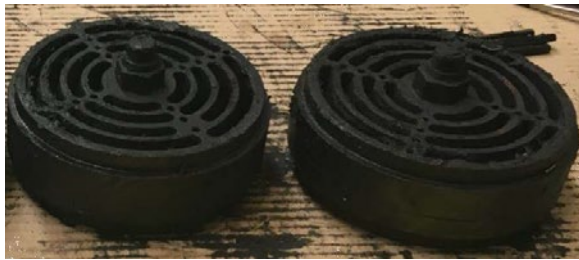
Figure 20: Sludge build up on the compressor valves on a USLG recycle compressor.
