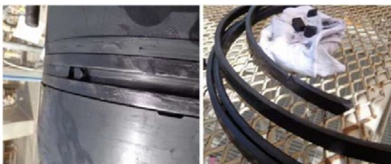
Figure 29: Broken piston rings
