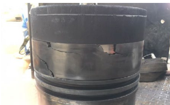
Figure 23: Piston with a broken rider band.
