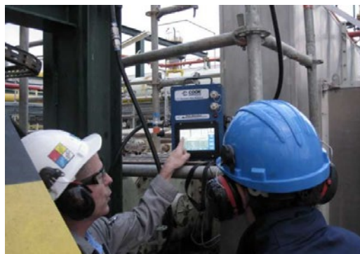
Figure 1: On-site flow measurement and analysis using a portable thermal mass flow meter
