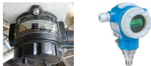
Figure 20: L.H.S: Digital Switch (to send inputs to digital boards), R.H.S: Pressure transmitter (to send inputs to Analog boards)
