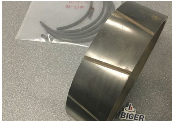
Figure 11: One rider band on the SW cylinder was cracked, the other one was worn but mostly undamaged.
