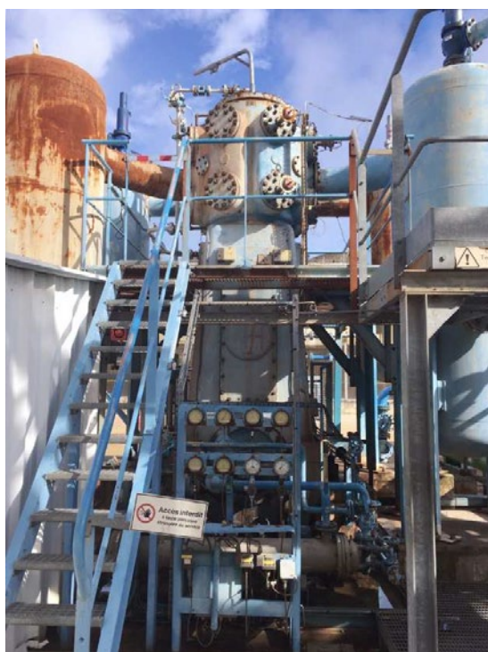
Figure 3: Compressor C02 at the operators plant. The first-stage cylinder head is at top centre. Two of the suction valve covers are visible, with their original pneumatic actuators; there are six suction and six discharge valves in total. The second-stage cylinder is behind, and the motor behind that.
