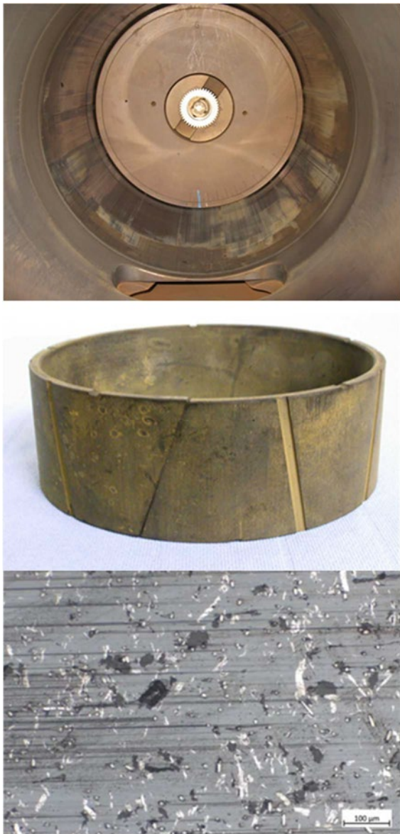
Figure 4: Ochre-coloured deposits in the compression chamber (top) and on a rider ring (centre), as well as the resultant abrasive wear in a piston ring's friction surface (bottom)
