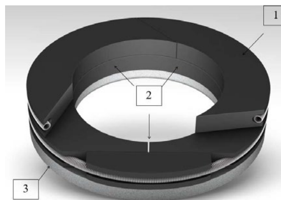
Figure 4: GTRS-Design with tangentially cut 3-piece design (1), a single cut sealing ring with a single cover segment (2) and a backup ring (3)
