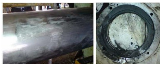
Figure 17: rubbed piston rod and damaged partition packing
