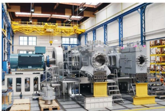
Figure 1: Three-stage compressor for compression of 70,386 Scm/h hydrogen to a final pressure of 154 bara for a refinery application
