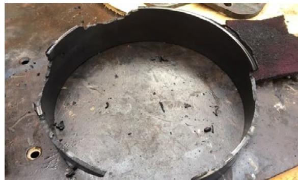
Figure 22: Rider band showing signs of extrusion (which indicates heavy blow-by) and breakages.
