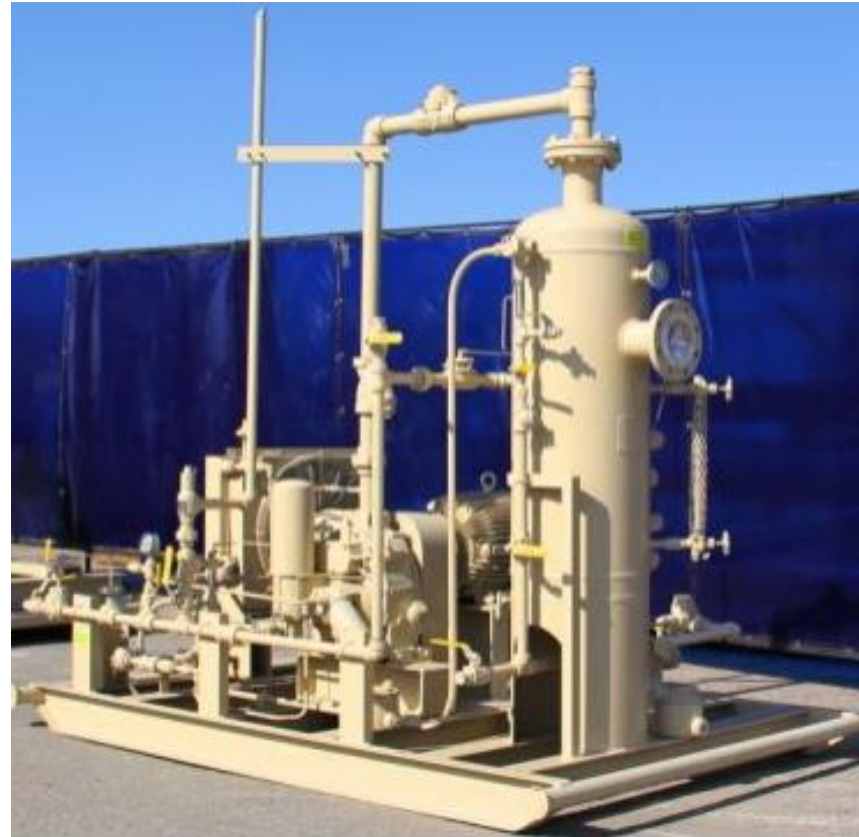
Photo of a typical VRU (source: HY-BON/EDI)
