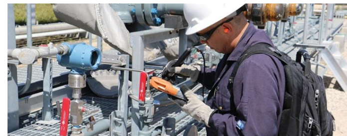
Example of a electronic sniffer screening
