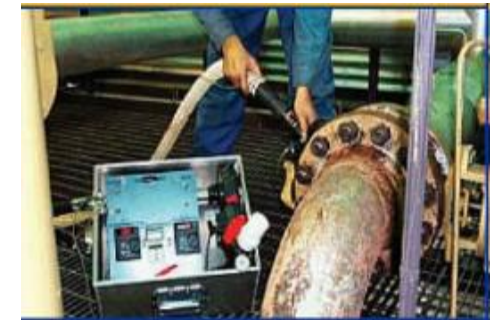
Example of bottom-up leak measurement using a high volume sampler
