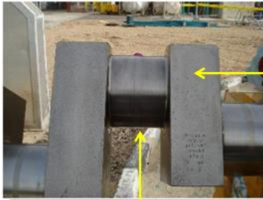
Crank Pin Bearing Journal Damage
