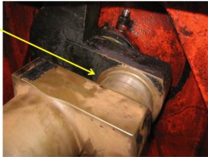
Crank Pin Bearing Journal Damage
