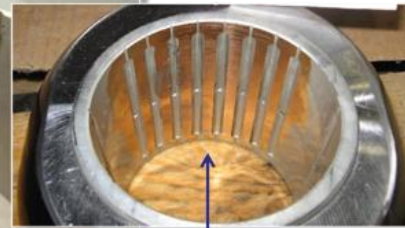
Obvious Wear Pattern; Still o.k. if Surface is smooth and Bearing ID within Spec.
