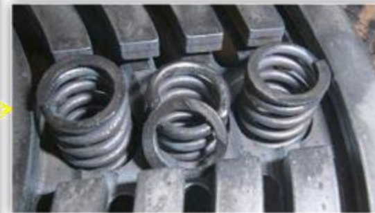
Slack and/or broken Valve Springs
