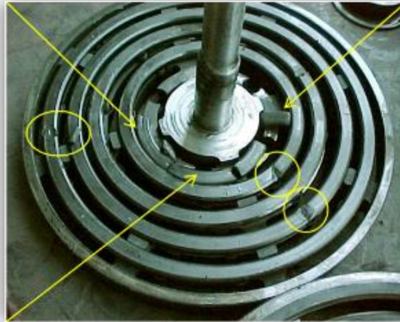
Cleaned for Photo Shooting Some Rings broken in various Pieces
