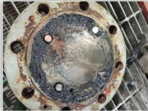
Piston Ring Wear "Mud" On Inside Valve Cover Surface
