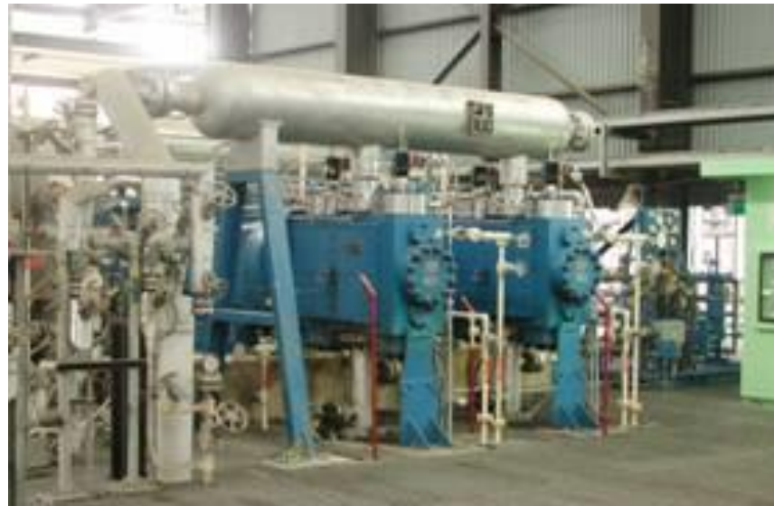
Recycle Side: 3rd-stage cylinders of a Mitsui C454 compressor equipped with HydroCOM, discharge pressure 203 bara
