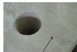
In case of cracks check if only from curing at the top surface or deep through the block
