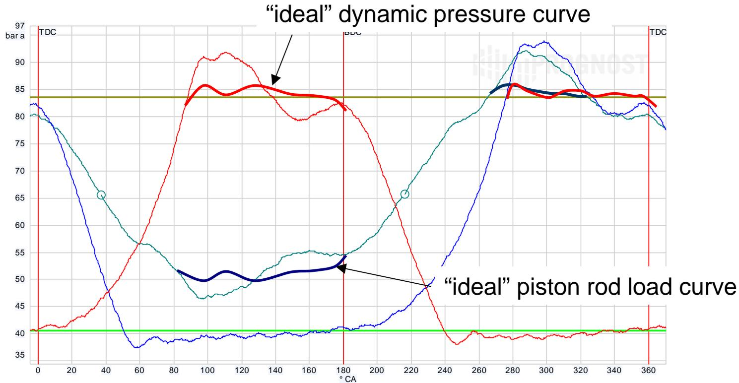
With "ideal" dynamic pressure curves (red) the resulting alternating piston rod load (blue) during the discharge phases would be significantly reduced.
