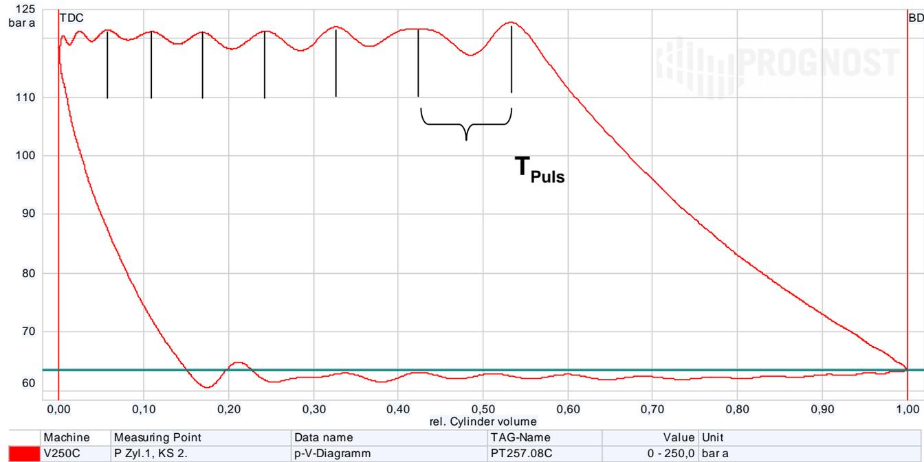
When displayed in a p-V diagram the same pressure pulsations often are not recognized as pipe pulsations, because they appear to have changing frequency.
