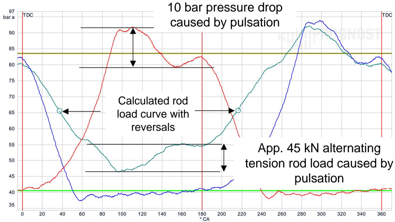
The pulsation in the discharge piping is causing a pressure drop of more than 10 bar during the discharge phase of the head and crank end compression chamber. This causes an alternating tension rod load of app. 45 kN, equivalent to app. 50% of the total tension rod load.
