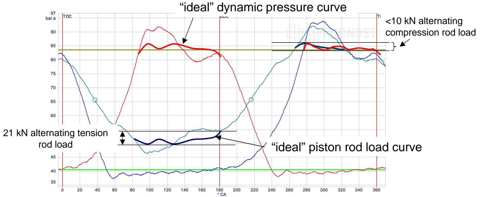
With "ideal" dynamic pressure curves (red) the resulting alternating piston rod load (blue) during the discharge phases would be significantly reduced by 20% of total tension rod load to app. 21 kN during tension phase and by 25% of total compression rod load to less than 10 kN during compression phase.
