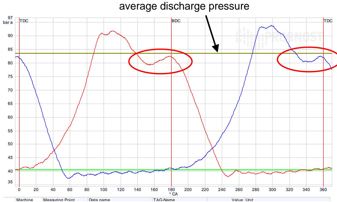
In the above example the pulsation in the discharge piping is causing the pressure in the cylinder even to drop below the average discharge pressure. This causes a significant change to the rod load as compared to ideal pressure curves.
