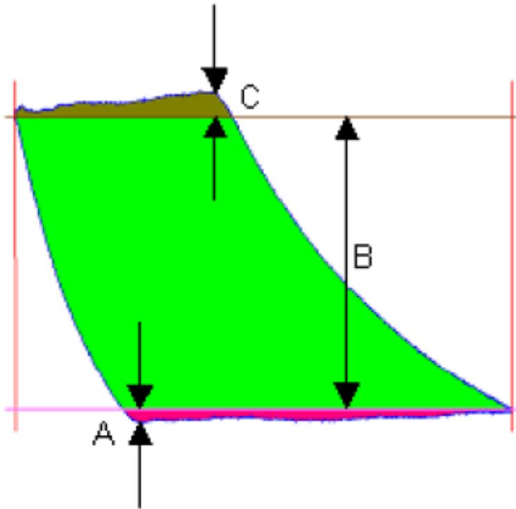
The valve inertia is a parameter that reflects the ratio of maximum pressure over- / undershoot of the dynamic pressure to the discharge/suction pressure (A or C) with regard to the pressure ratio (B). An increasing valve inertia indicates a rising pulsation or delayed opening of the suction/discharge valve.
