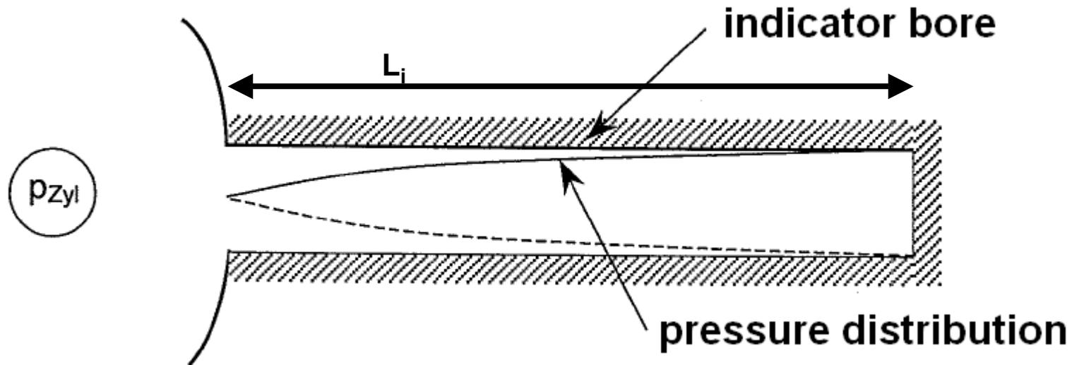
The channel resonance is an **acoustic effect** that results from the **length of the indicator tap** and the **speed of sound**. It causes a **pressure pulsation** on the dynamic pressure signal that might be **mistakenly** considered a pressure pulsation. It has to be **eliminated** from the signal by an appropriate **low-pass filter**.
