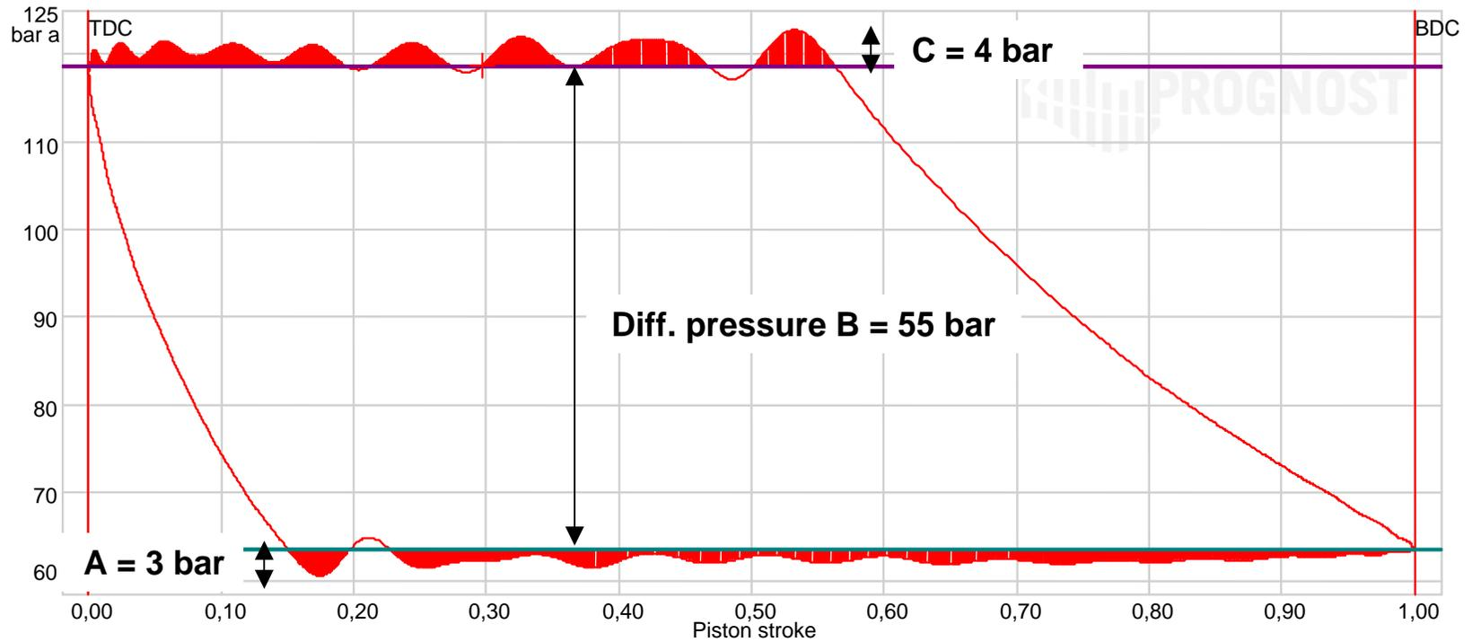
$$\text{Inertia discharge} = C / B = 4 \text{ bar} / 55 \text{ bar} = 0,073$$
