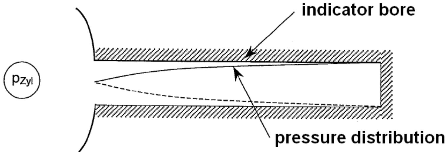
Examples : Calculated channel resonance for indicator tap length 450 mm at 20 °C
