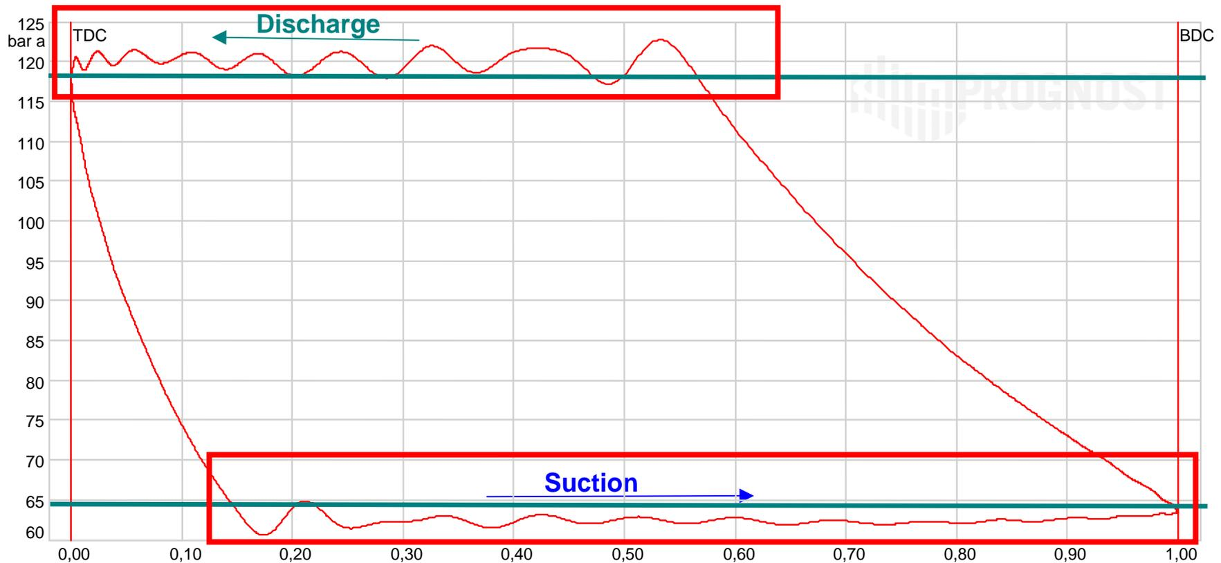
The pulsations in the suction and discharge piping can be monitored by the dynamic pressure measurement e.g. as a p-V diagram during the suction and discharge phase. However, this is only an indirect measurement and does not represent the real magnitude of pulsations in the piping.
