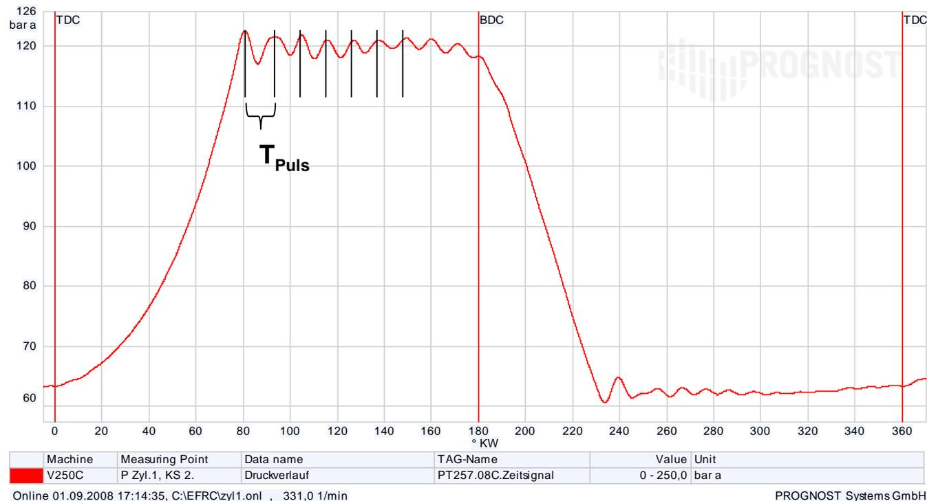
Pulsations can best be viewed in time related dimensions that illustrate the stable frequency of pulsations. Often mistakes are made when pulsations are judged by watching p-V diagrams that are using a volume dimension on the horizontal axis.
