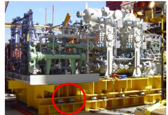
BLOCK OR MACHINE MOUNTED ON ANTI VIBRATION MOUNTS (AVM'S)
