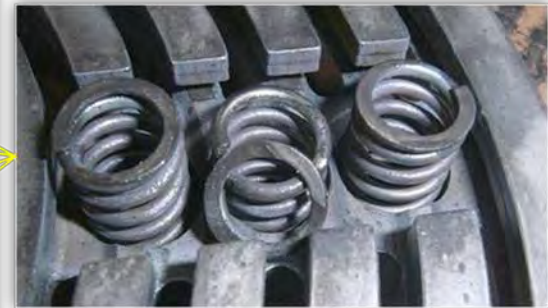
Slack and/or broken Valve Springs
