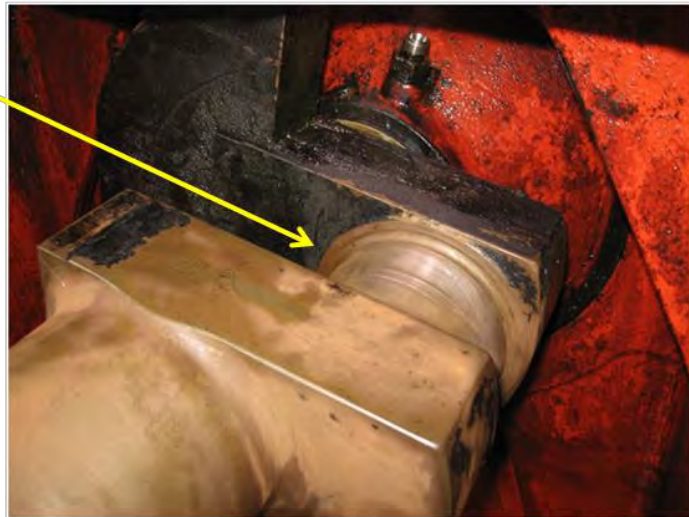
Crank Pin Bearing Journal Damage
