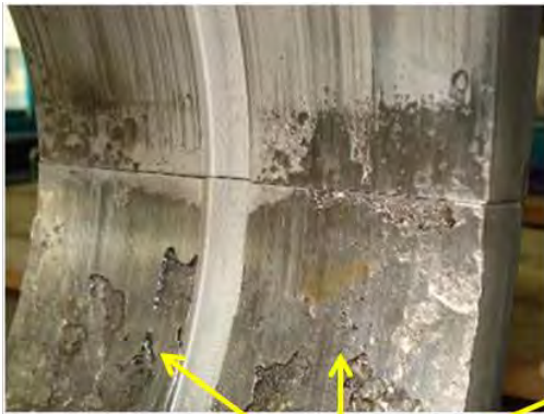
Crank Pin Bearing Damage
