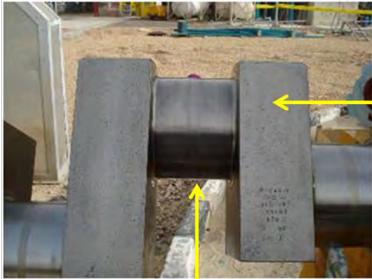
Crank Pin Bearing Journal Damage
