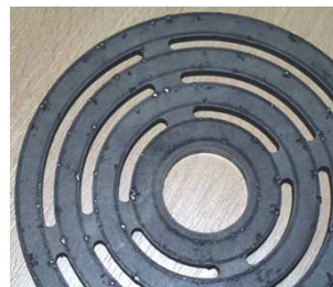
Plastic valve plate with embedded particles
