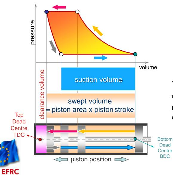
Volumetric efficiency  $\eta_v = \frac{\text{suction volume}}{\text{swept volume}}$
