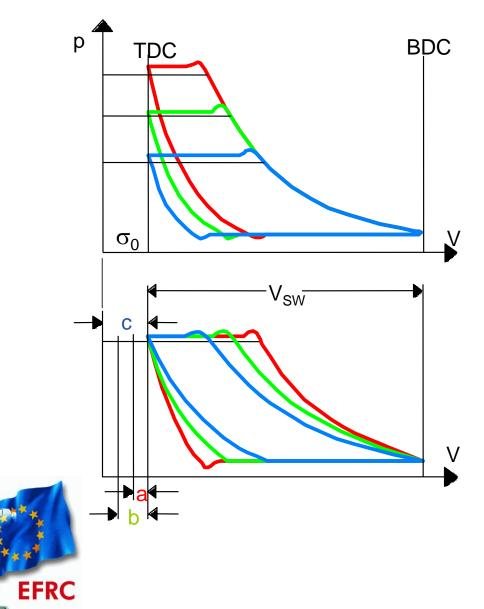
Influence of pressure ratio p2/p1 on volumetric efficiency:
