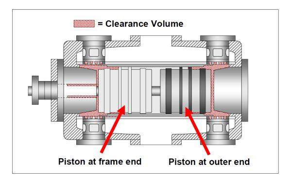
•Clearance refers to the volumes in each end of the cylinder that retain gas after the piston has stopped
