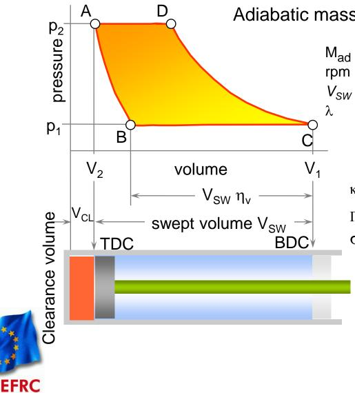
Adiabatic mass flow  $M_{ad} = \rho_s V_{SW} \lambda^* rpm/60$
