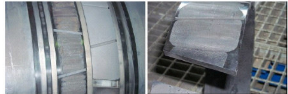
Figure 5: Photographs showing the wear pattern of the rider rings.
