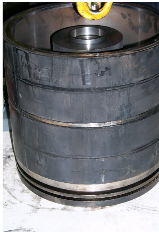
Figure 8: damaged rider rings 1st stage
