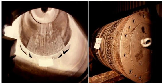
Figure 4: Photographs of the damage on the liner after mechanical contact
