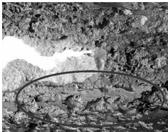
Figure 3: Corrosion attack at the damage point
