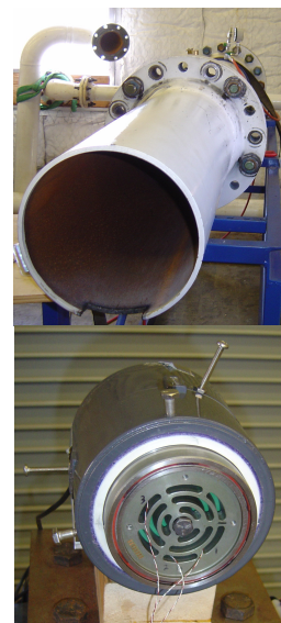
Figure 4: Burst-Membrane Shock-Tube (Top) and Instrumented Valve Fixture (Bottom)
