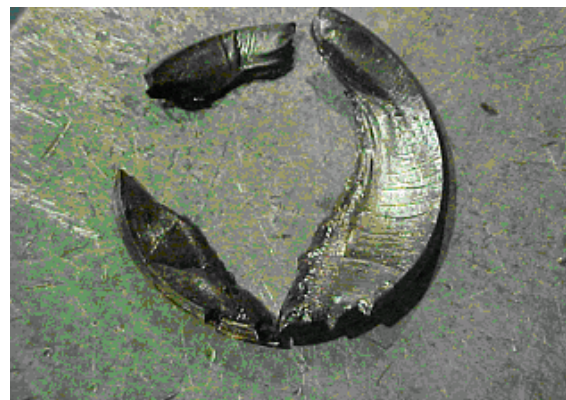
Figure 5: Fragments of the piston rod thread region
