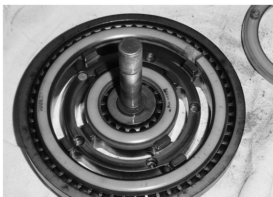
Figure 5: Cylinder 5 HE suction valve 1 with liquid slugging damage (oil and condensate)
