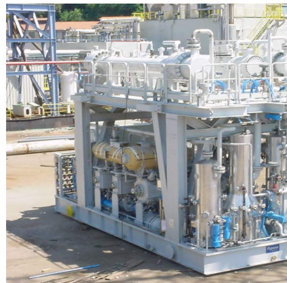
Figure 5: One of the four MP/HP compressor packages. L \times W \times H = 10.5 \times 4.7 \times 6 meter and an operational weight of 150 tonnes.
