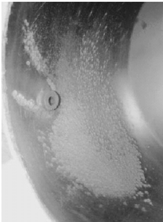
Figure 17: Aerial excavation on the jacket
