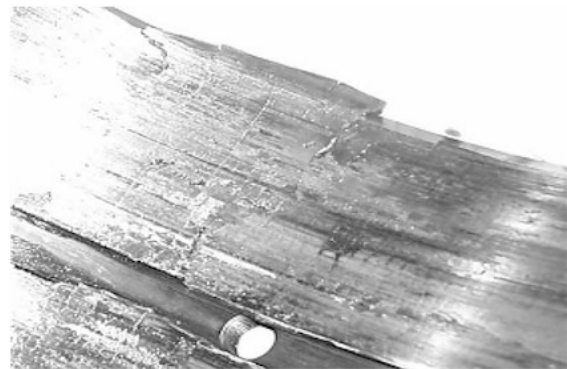
Figure 7: One of the cylinder 6 bearings that failed in 2000
