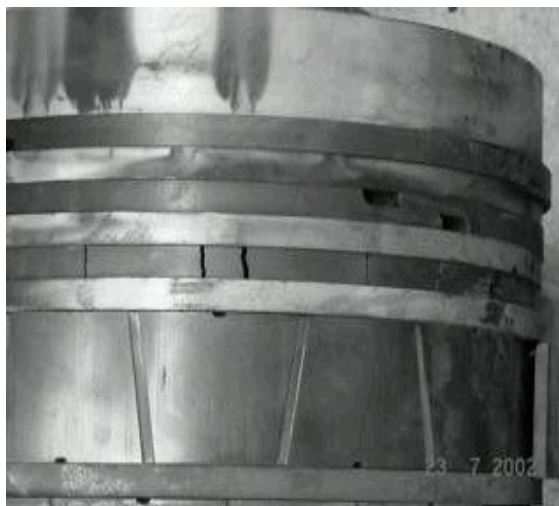
Figure 3: 2 nd stage piston showing significant wear and tear at piston and rider rings also scratch marks there piston touched the cylinder liner
