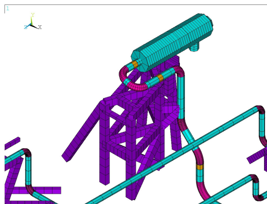
Figure 11: Support suction side 1 st stage modified by TNO
