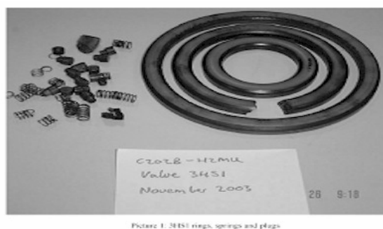
Figure 15: 3HS1 valve internals
