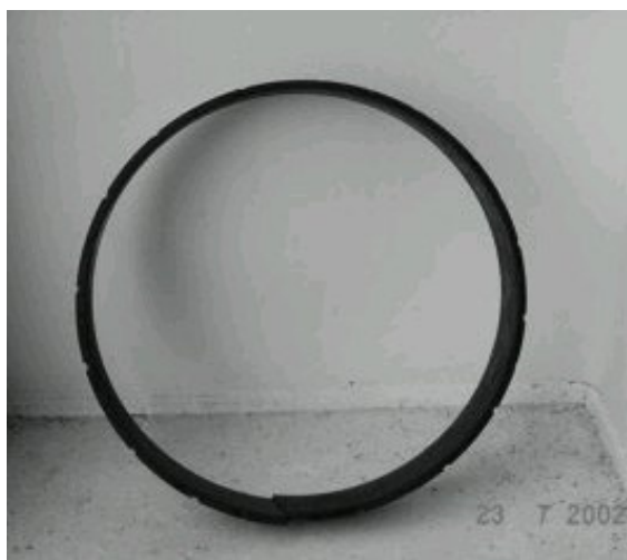
Figure 4: 1st stage rider ring showing significant localized loss of thickness
