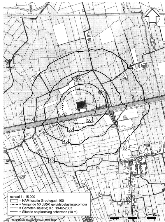
Figure 2: Original noise contour as determined by an independent acoustic consultancy firm [1]; the dotted line indicates the permitted 50dBA noise contour
