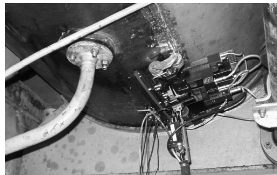
Figure 18: Ultrasonic scanner at 06-00-h position
