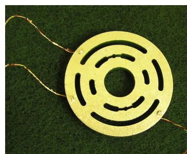
Figure 5: Valve Plate with Reflective Coating and Mounted Strain Gauges
