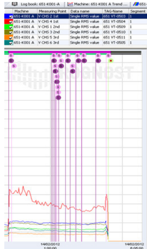
Figure 6: Trend view of the vibration RMS analyses of all six crosshead slides of the compressor
