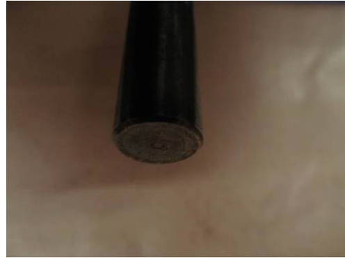
Figure 13: No wear on the actuator rod after 8000 running hours.
