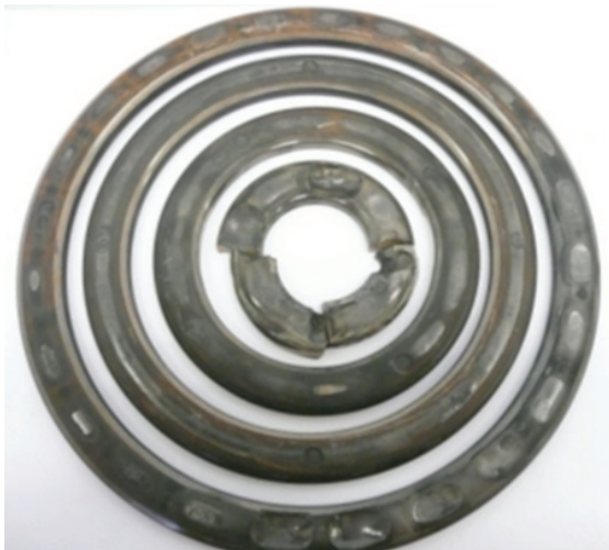
Figure 2.3: Case 2: Damage with too little control pressure
