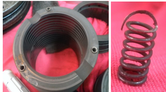
Figure 7: Labyrinth Packing Ring and Damaged Spring
