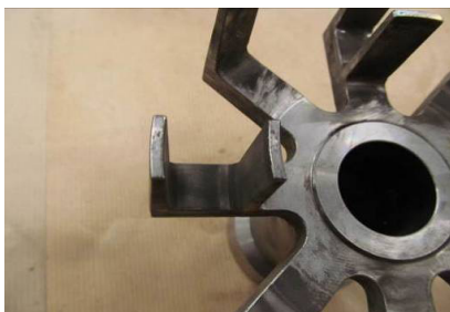
Figure 12: No wear on the fingers after 8000 running hours.
