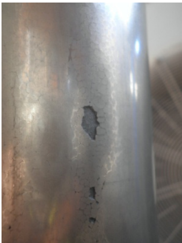
Figure 6: Damaged Piston Rod
