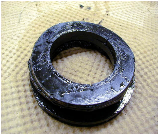
Figure 6: Reciprocating compressor packing case rings with signs of excessive lubrication.
