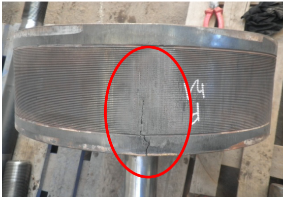
Figure 2: Damaged Labyrinth Piston
