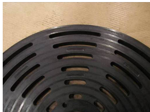
Figure 14: Slight signs on the plate produced by the fingers which didn't have any effect on regulation.
