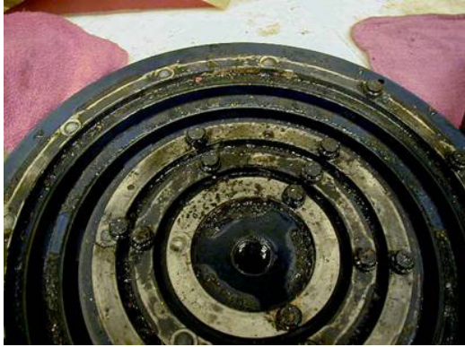
Figure 5: Reciprocating compressor valve with signs of excessive cylinder lubrication.
