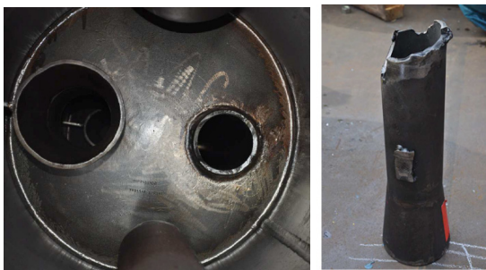
Figure 6 Broken baffle choke tube of discharge 1 st stage damper (inlet side)
