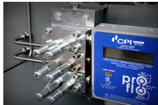
Figure 4: Divider Block component with lubrication monitor and shut down device
