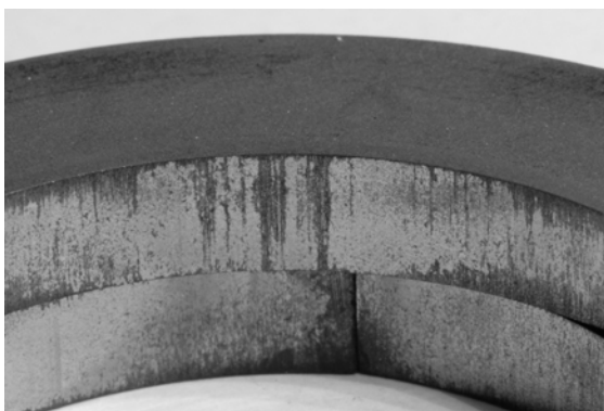
Figure 10: Silver-coloured layer on the friction surface of a dry-running packing ring after operation on a CrC/NiCr-coated piston rod
