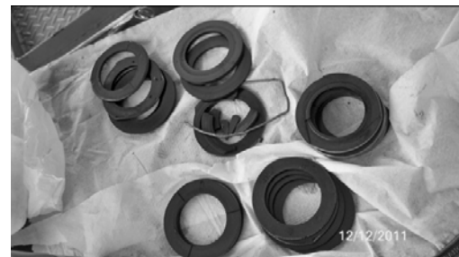
Figure 12: Packing ring set – shows broken spring and packing rings
