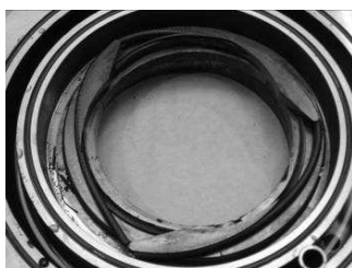
Figure 19: Failure of the sealing elements in the pressure packing
