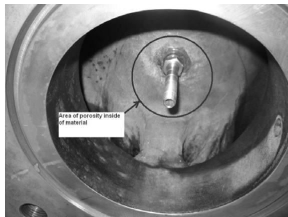
Figure 2.4.1.6: Porous area - cast cylinder - St. 3
