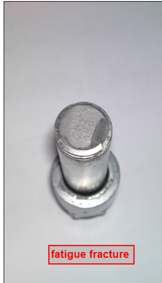
Figure 5: broken stud bolt fracture surface
