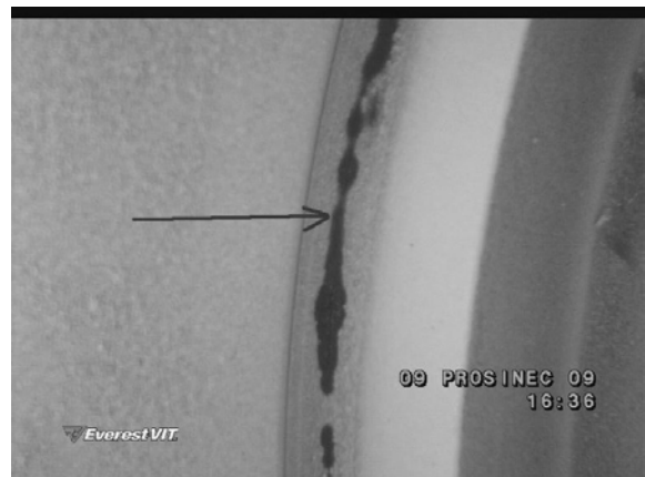
Figure 2.4.1.2: Circumferential valve seat crack
