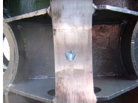
Picture 29: old frame showing connection bolt hole not in the middle
