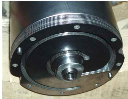
Figure 3.4: Package of guidance springs mounted on magnet
