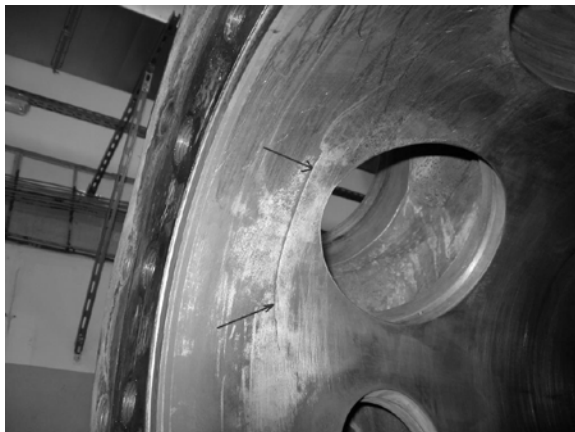
Figure 2.4.1.3: Crack propagated into cyl. bore
