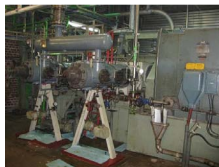
Picture 33: with new frame housing and cylinder supports
