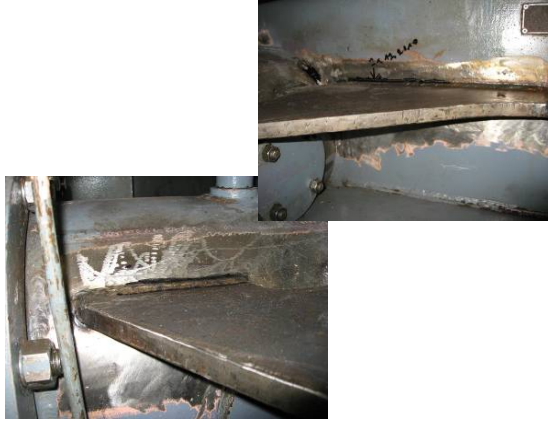
Picture 8+9: New welding were indicating former cracks
