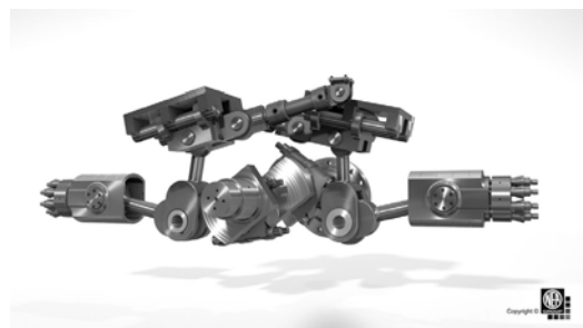
Figure 13: Linkage design of variable stroke flow control
