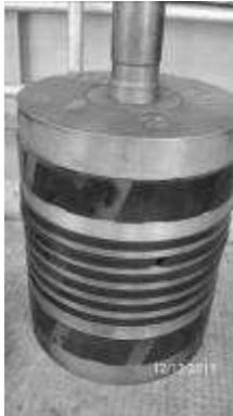
Figure 7: Campana hydrogen compressor piston after 9300 hours of operation
