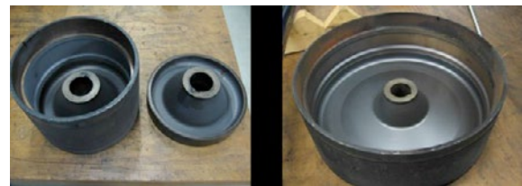
(Fig. 25) original 2 nd stage piston (Fig. 26) original 1 st stage piston
