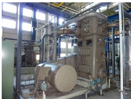
(Fig. 31) The CO 2 compressor operating after the modification of both pistons
