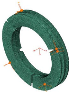
Figure 2: RT ring pair showing positions of the artificial springs that prevent the segments from rotating.
