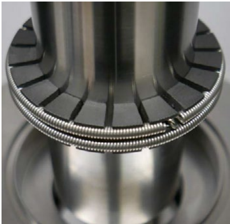
Figure 14: 20-piece ring mounted on the rod of the friction test device.
