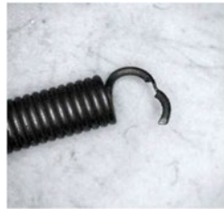
Figure 2: Damaged spring eye leading to spring failure
