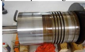
(Fig. 12) modified piston
