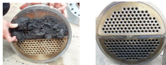
Figure 5: Heat exchanger before and after changing to PAG based compressor oil
