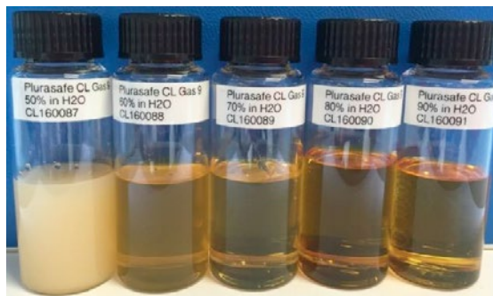
Figure 3: Water-soluble compressor oil with contamination of 10% to 50% of water
