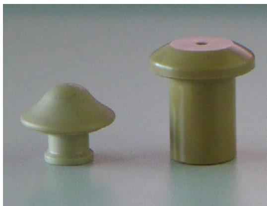
Figure 2.8: Comparison of a standard to an Arrowpoppet of nominal size (i.e. the diameter of the bore in valve seat) = 20 mm
