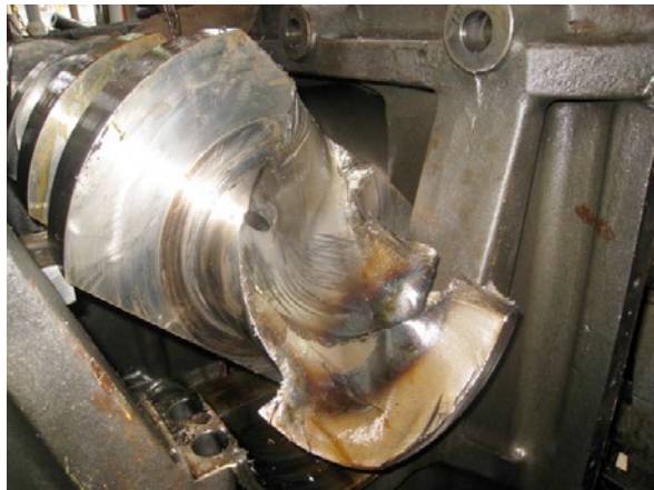
Figure 7: Torsional failure of a compressor crankshaft.
