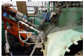
(Fig. 9) drilling of lube connections
