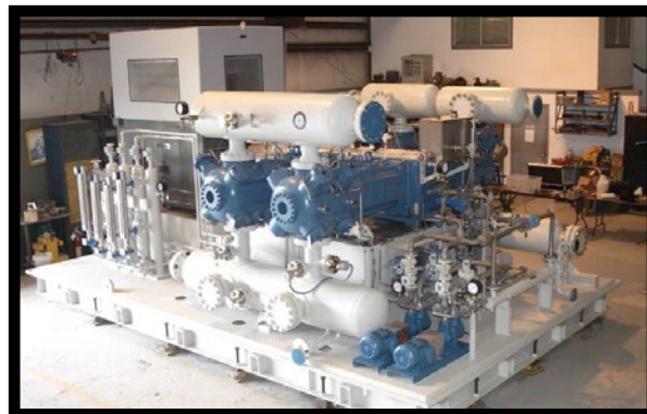
Figure 3: Compressor package showing vent and drain collection pots.
