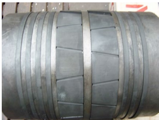
(Fig. 6) Piston with extensive wear one middle sections of the rider rings
