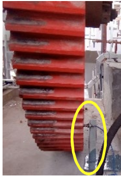
Figure 4. Flywheel Top Dead Centre Sensor TDC used in the capacity control system.
