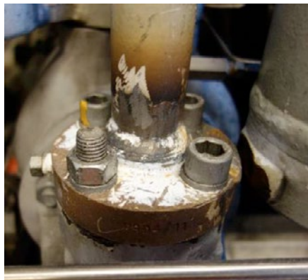
Figure 4: The weld history at the 4th stage suction cylinder connection.
