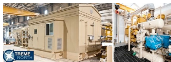
Figure 8: Cold weather compressor package showing the skid and the inside of the skid mounted building. 1
