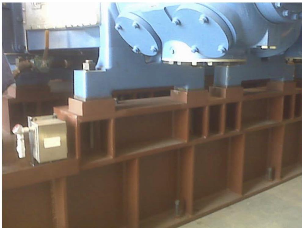
Figure 12.3 Well-designed crosshead guide supports provide high axial (parallel to the crankshaft) and vertical stiffness that usually eliminates the need for head end cylinder supports [7]
