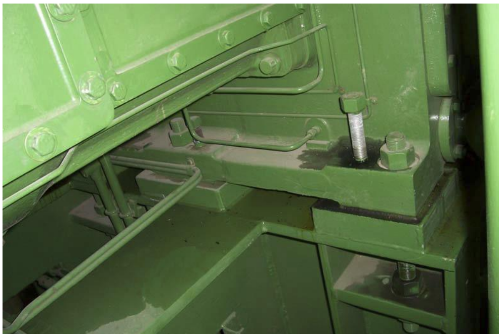
Figure 11.15 Example of achieving extended length of crosshead guide anchor bolts, including horizontal reinforcing plate [6]
