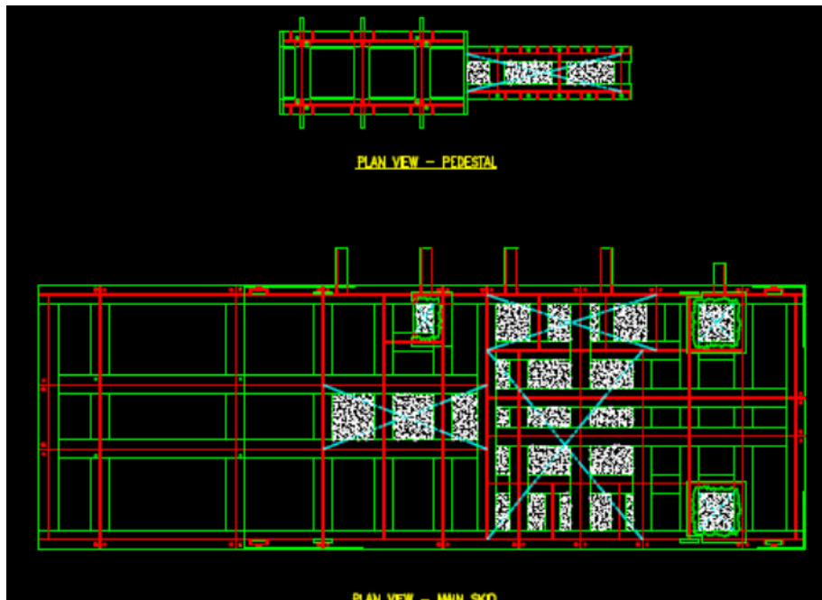
Figure 11.9 Typical skid showing concrete fill locations [7]
