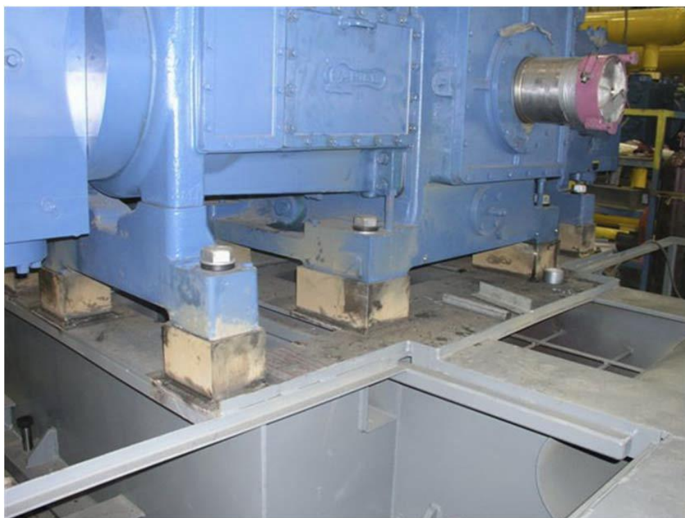
Figure 12.15 Welded steel chock (shall be machined after welding) [7]
