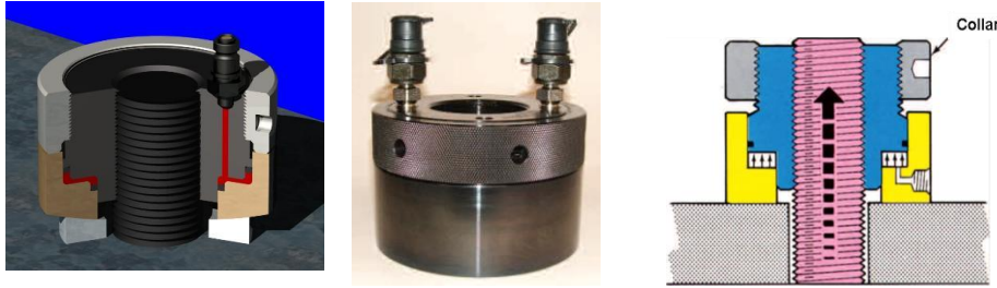
Figure 8.9 Working principle of a hydraulic nut
