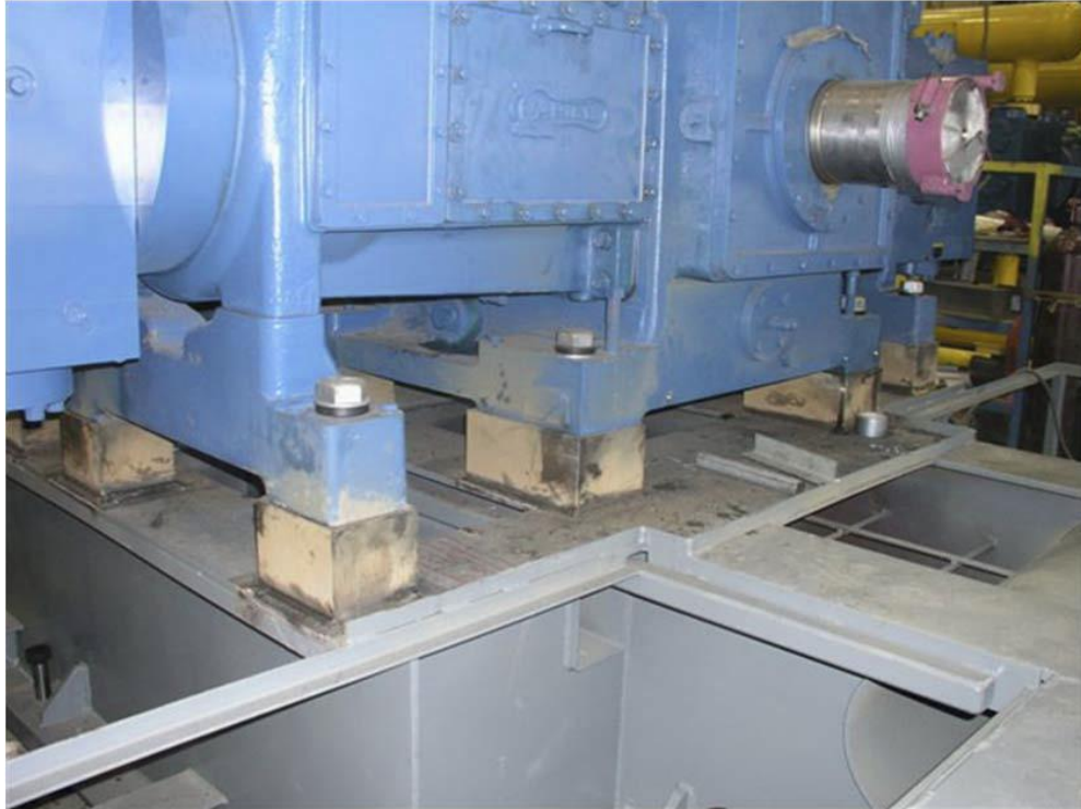
Figure 12.2 Welded steel chokes shall be machined after welding [7]
