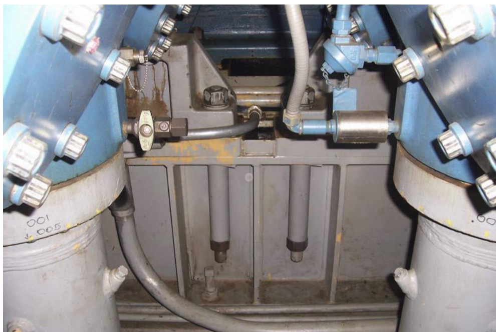
Figure 11.13 Example of achieving extended length of crosshead guide anchor bolts [6]
