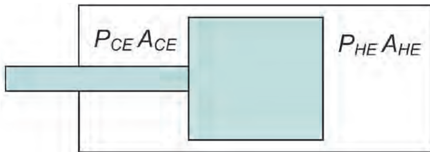
Figure 1. Diagram for calculating gas load on the piston.
