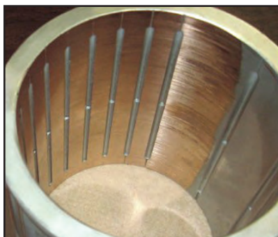
Figure 6. Connecting rod bushing configuration A corresponding to the loading diagrams in Figure 5a, showing heavy wear on the crank-end side after a short period of operation.
