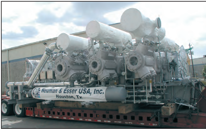
■ The medium-speed six-crank SSL320hs compressor.
