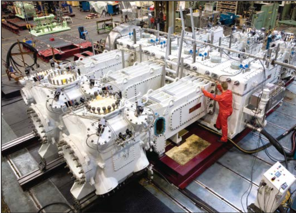
■ A C-85.6 is shown here undergoing its API test at the Thomassen premises in Rheden, Netherlands. The API 618 range of reciprocating compressors is seven strong, ranging from the C-7 model with a maximum power of 1070 hp (800 kW) at a rated speed of 600 rpm, up to the largest — the C-85.
